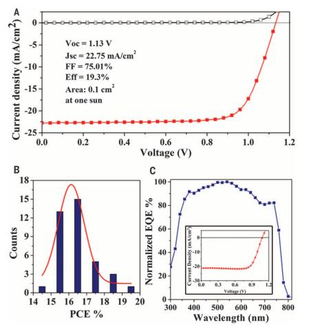
Fig. 3. Efficiency measurements. (A) J-V curves for the champion cell without antireflective coating. (B) Histogram of solar cell efficiencies for 40 devices. (C) Normalized EQE spectrum of a typical cell. (Inset) The corresponding J-V curve of the device.
